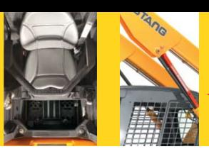
Fluid fill points and filters are all readily accessible, and air cleaner inspection is simplified with a visual air restriction indicator.
