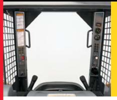
The Mustang ROPS/FOPS lifts up effortlessly, providing the service technician with easy access to the hydrostatic pumps.
