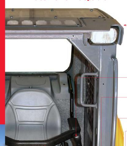
The Mustang skid-steer features a spacious ROPS/FOPS Level II - certified operator compartment
